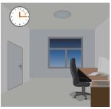
Light will switch off after the hold time when no movement in detection area.
