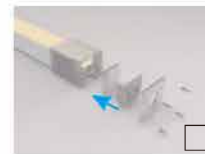
put waterproof pad, PC pad and metal pad then fixed by screws
