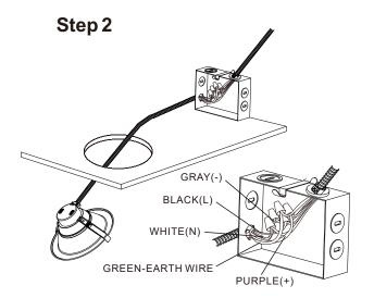
Connect AC and Dimming wire correspondingly as shown in picture
