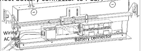
Step 3: Push the unit back to the junction box, assembly panel module.
