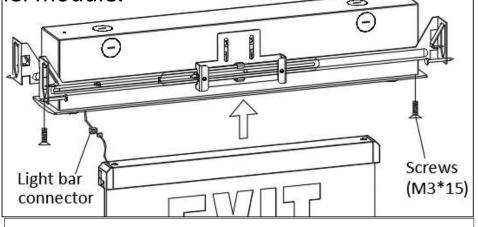
Step 4: ceiling or surface mount for panel module.
