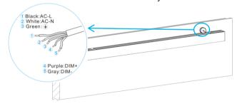
Explain: connect to ①、②、③ only if do not need to use dimming function, no need to connect ④、⑤
