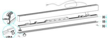
(4) Assemble carrier, diffuser and anti-lightleak clips
