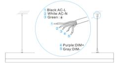
Explain: connect to 1, 2, 3 only if do not need to use dimming function, no need to connect 4, 5
