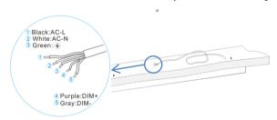
Explain: connect to ①、②、③ only if do not need to use dimming function, no need to connect 4, 5
