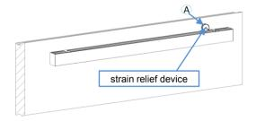
Note: (A) outlet box and strain relief device (prepare by user)
