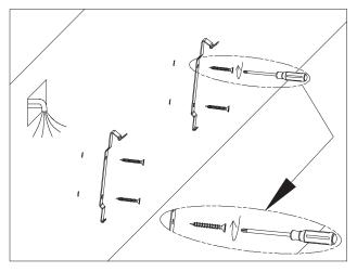
3. Thread screw through clamp, and fasten the clamp into plastic rubber with cross screw driver, and draw out AC input wire from junciton box in wall;
