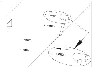
2.Drive the plastic rubber into 4 holes of  $\varphi$ 3.0mm with hammer, and thread screw through fixed head 2,then fasten fixed head 2 into plastic rubber with cross screw driver and insert junction box into wall;
