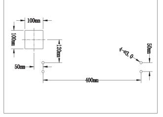
1. Drill 4 holes of  $\phi 3.0mm$  and 1 hole for junction box;
