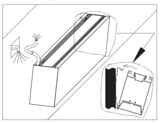
4. According above detailed drawing, install lamp on one side of clamp, and rotate lamp to other side of clamp;
